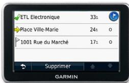
Coupled with the Astus Tag module, the Garmin navigation screen becomes a multi-purpose messaging tool. Unique features are added to the basic GPS functions: real-time communication between the manager and the drivers, task-dispatching, route planning with estimated time of arrival.
