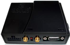
Our main product, the Astus Tag module, is an electronic box which records its position by GPS at specified intervals or on change of position, as well as other data like speed and distance traveled. The information is transmitted through the cellular network and can be viewed and analyzed with our Astus software.
